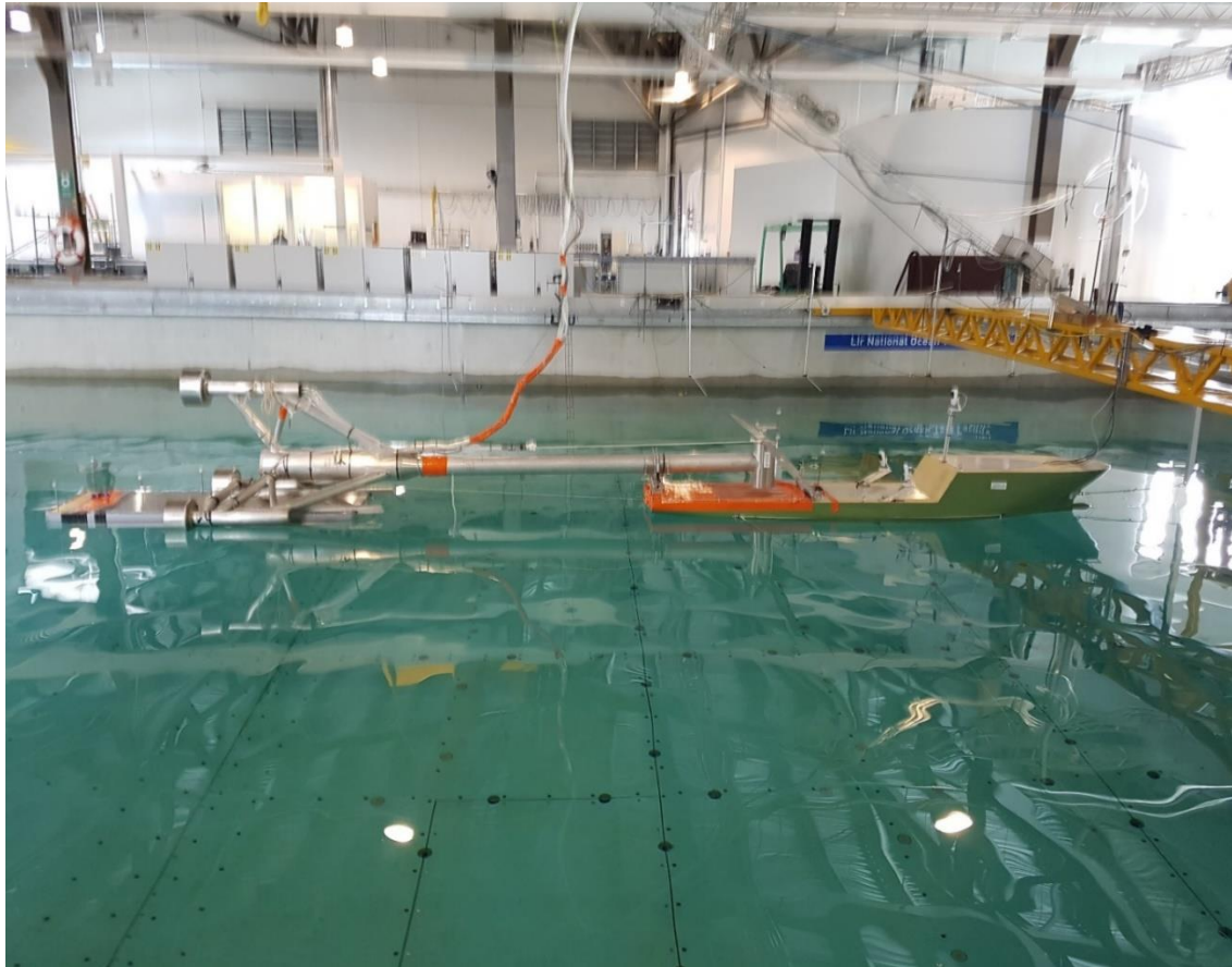
Figure 4. Arrangement of test facilities for the testing of the MINT transport and installation method for wind turbines.
